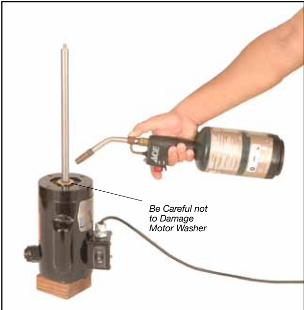
Fig. 23. Place Motor/Shaft Assembly on Stand. To activate Loctite adhesive, torch Shaft about 2 to 3 inches (50 to 75 mm) above Motor for 7 seconds. Be careful not to damage Motor Washer. Allow Shaft to cool.
