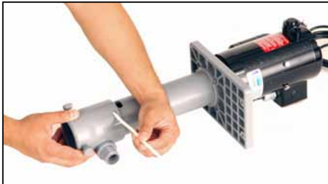
Fig. 35. Push Teflon Strap into hole while turning Swiveling Impeller Housing back-and-forth. Teflon Strap secures Swiveling Impeller Housing to Body.
