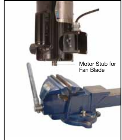
Fig. 17. Tighten bench vice onto Motor Stub, where Fan Blade is normally mounted. Make sure Motor is firmly secured.
