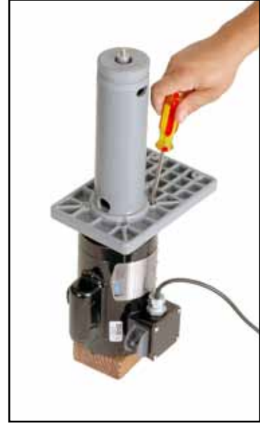
Fig. 30. Use Phillips-head screwdriver to tighten screws onto Pump/Motor Base, through Spacers and into Motor.
