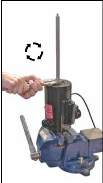
Fig. 22. Secure Motor on bench vice. Screw long Shaft onto short Motor Shaft. Tighten clockwise with vice grips.
