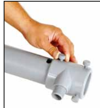
Fig. 36. Rotate Swiveling Impeller Housing to desired position for installation in tank, then tighten Lock Screw.
