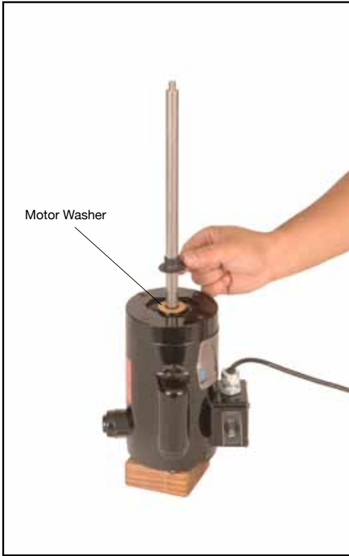
Fig. 24. Proceed with this step only after Shaft is balanced. With Motor off, push Boot Seal onto Shaft until it touches Motor Washer.
