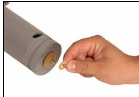
Fig. 32. Push Impeller Washer over threaded Shaft until flush against Super Slinger. Make sure Impeller Washer lays flat.
