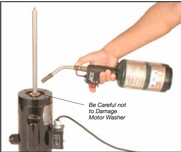
Fig. 18. Torch Shaft for 20 seconds about 1 to 2 inches (25 to 50 mm) above Motor to loosen Loctite adhesive. Be careful not to damage Motor Washer.
