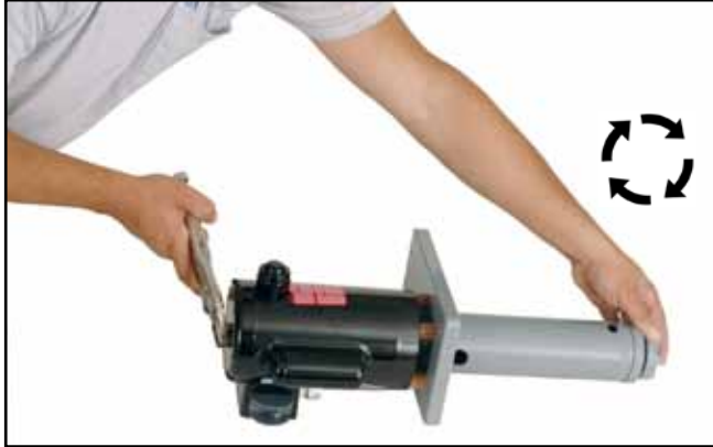
Fig. 33. Install Impeller. While firmly holding Motor Stub with vice grips, turn Impeller clockwise with hand. Impeller should spin freely and not touch pump body.
