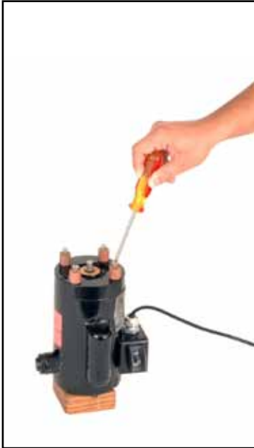
Fig. 20. On new Motor, use Phillips-head screwdriver to remove four screws holding Spacers. Set Spacers aside.
