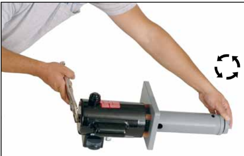
Fig. 11. While firmly holding Motor Stub with vice grips, turn Impeller counterclockwise with hand.
