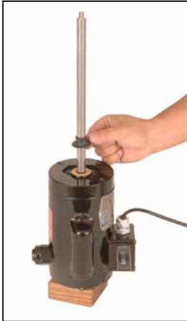
Fig. 16. Remove Boot Seal and set aside for reuse. Or order a new Boot Seal if old one is badly worn or damaged.
