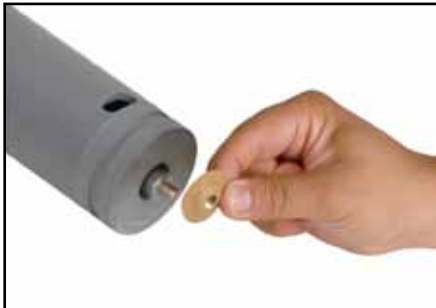
Fig. 31. Push Super Slinger over threaded end of Shaft. Note that flat side of Super Slinger must be against pump body.
