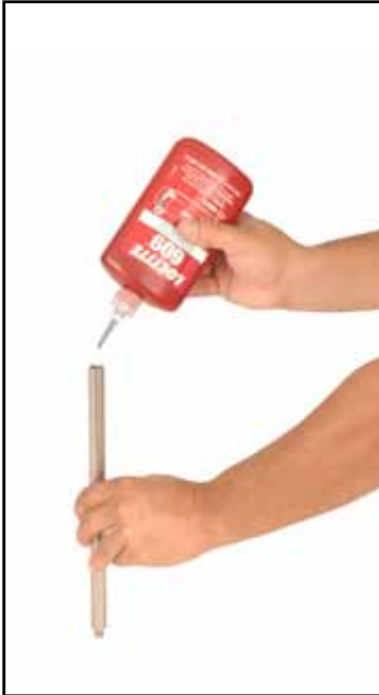
Fig. 21. Apply a drop or two of Loctite inside female threaded end of Shaft that screws onto Motor.
