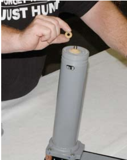
20. Install Impeller Washer (in hand) over Super Slinger.
