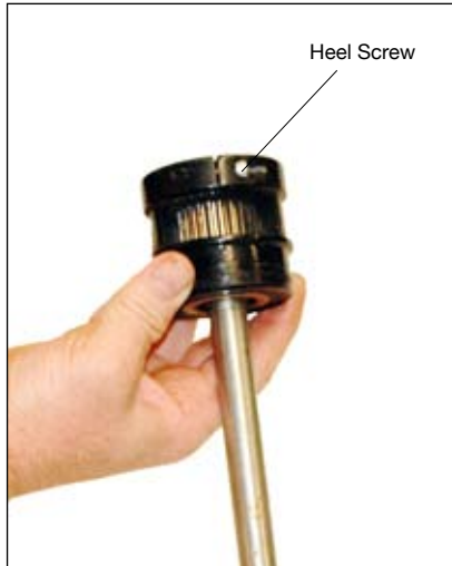
7. Loosen Heel screw with 5/32" Allen wrench.
