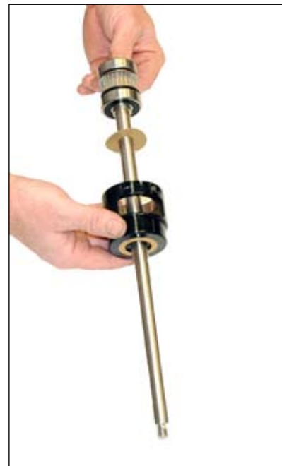
10. View of Shaft Bearing Assembly separated from Heel.
