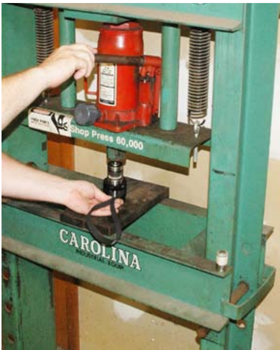
13. Use Machine Press to complete installation of Shaft Bearing Assembly into Heel.
