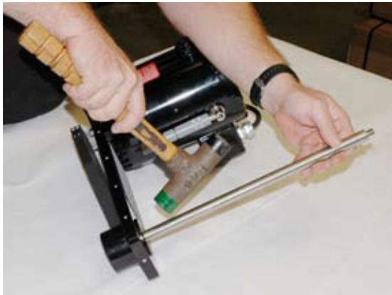
5. (Above) Use mallet to break seal around Heel.
