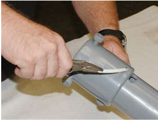
1. Remove Teflon Strap from Impeller Housing.
