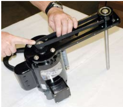
16. Slowly "walk" belt onto motor pulley.
