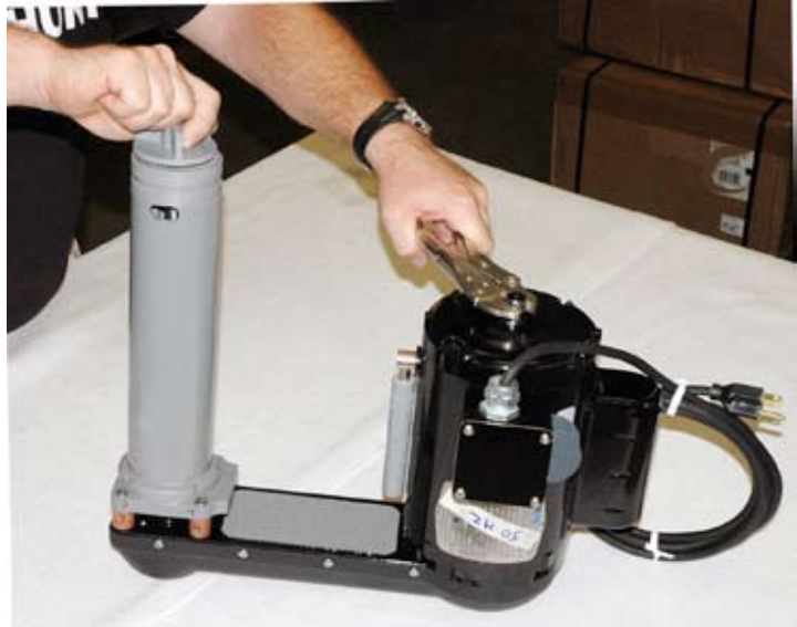
21. While holding Fan Blade end of shaft with vice grips, tighten impeller by hand.
