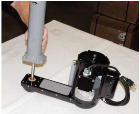
19. Make sure Spacers are in correct numerical position (refer to Fig. 3), then install Pump Body/ Pump Base assembly.
