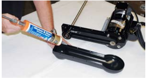
17. Apply silicone sealant to Belt Drive Cover.
