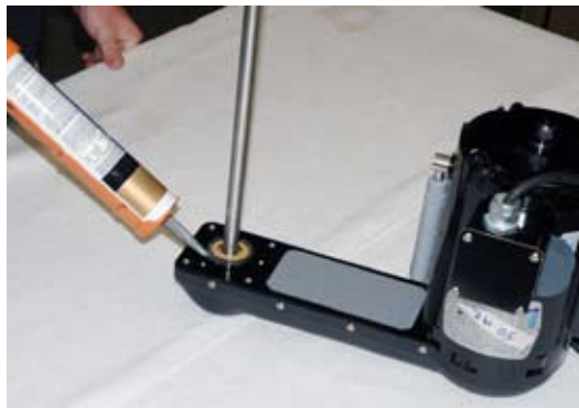
18. Apply silicone sealant around underside of Heel.
