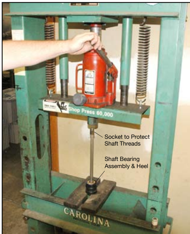
9. Remove Shaft Bearing Assembly from Heel with machine press.
