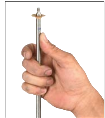
Fig. 5. With mark facing you, again place hand firmly on Motor and use other hand and thumb to push “high” spot on Shaft.
