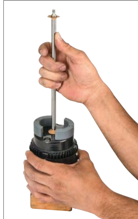
Fig. 2. For rough balancing procedure, put one hand firmly on Motor to stabilize assembly. With other hand, use hand and thumb to push “high” spot on Shaft.
