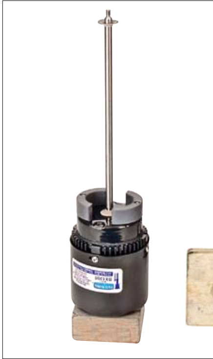
Fig. 1. Position pump on Motor Stand. Then hold Motor firmly with one hand and keep safe distance from Shaft. Turn Motor on briefly to observe Shaft. Caution: Shaft may swing wildly if badly out of balance!
