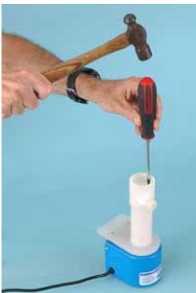
Fig. 3—Using hammer and blunt screwdriver, tap Flow Plate.
