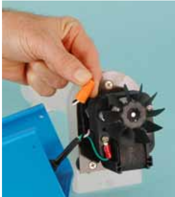
Fig. 8—Remove wire nuts and disconnect electrical wires on Motor.
