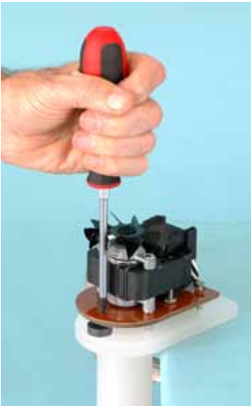
Fig. 16— Align Motor Plate holes with Spacer holes and Base holes. Tighten screws.
