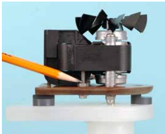
Fig. 18— If Shaft is not centered in hole, it may be necessary to adjust two hexhead Shaft Adjustment Screws that go from Motor through Motor Plate. Two open-end wrenches are needed—11/32" for the hex-head (top) and 1/4" for the hex washer head (bottom).
