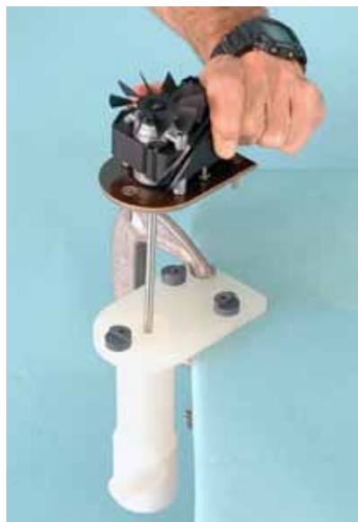
Fig. 12 —Lift Motor/Shaft Assembly to separate from Base, Body & Impeller Housing.
