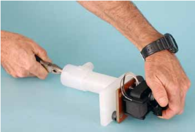
Fig. 10a—Hold Impeller firmly with needle-nose pliers while using cupped hand to gently turn Fan Blade counterclockwise. (As an alternative, use Allen wrench as shown in Fig. 10b.)
