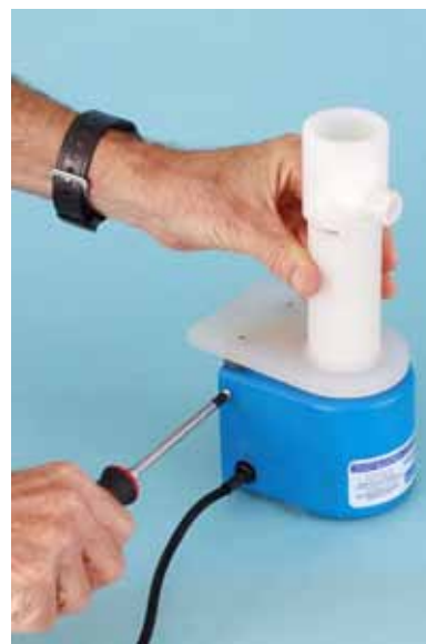
Fig. 5—Remove three screws from Motor Cover.
