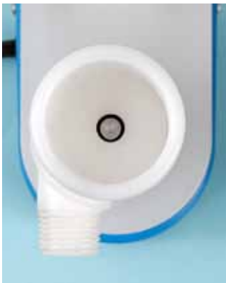
Fig. 17— Remove C Clamp and turn pump upside down. Look into Impeller Housing to make sure Shaft is approximately centered in hole, as shown. If properly aligned, ignore Fig. 18 and proceed to Fig. 19.
