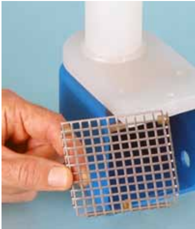
Fig. 6—Remove Screen from Motor Cover.
