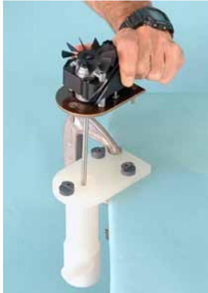
Fig. 15— Install new Motor/Shaft Assembly into pump body.
