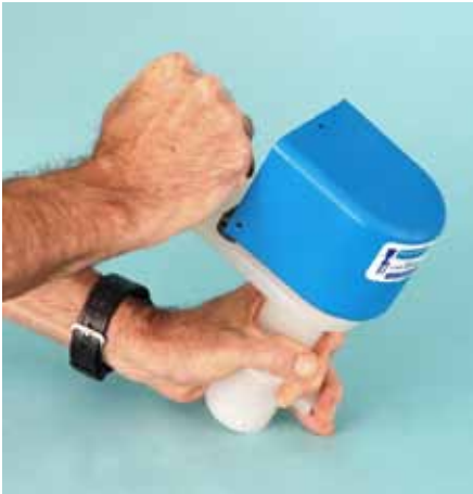
Fig. 7—Remove Motor Cover by sliding off or striking with hand.
