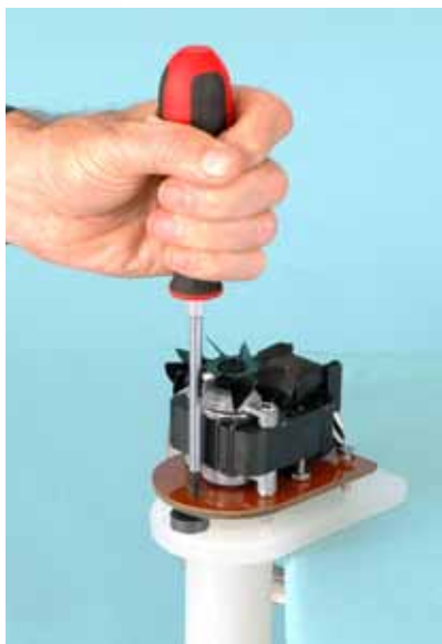
Fig. 11 —Secure pump on table with C Clamp. Then remove three flathead Phillips screws that hold Motor Plate to Pump Base.
