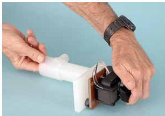
Fig. 19 —Hold Impeller firmly with fingers while using cupped hand to gently turn Fan Blade clockwise. When you feel resistance and Fan Blade begins to bend, that's tight enough. Alternatively, use a 3/32" Allen wrench to hold Fan Blade stationary while turning Impeller clockwise with fingers. Allen wrench opening is on Fan Blade hub, just beneath blades.
