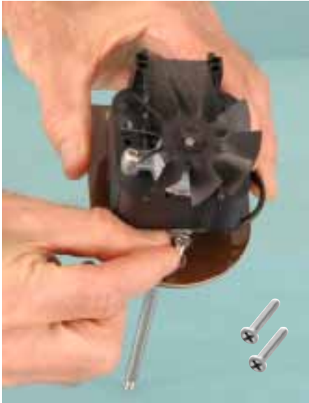
Fig. 14— Insert three 8-32 x 1" flat-head SS screws through Motor Plate on Motor/Shaft Assembly.
