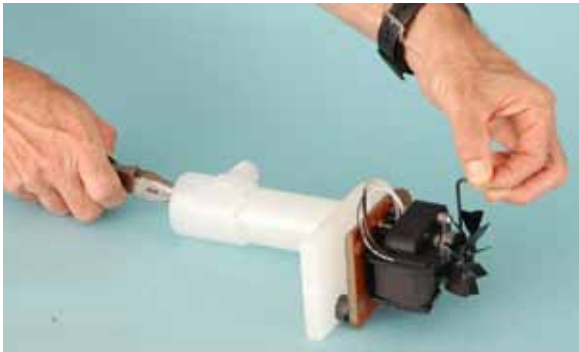
Fig. 10b—As an alternative to Fig. 10a, you can use a 3/32" Allen wrench to hold Fan Blade stationary while turning Impeller counterclockwise with fingers or needle-nose pliers. Allen wrench opening is on Fan Blade hub, just underneath blades.
