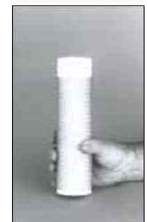
(L-r) Place plastic loading slats over filter. Then slide web over slats and pull down. Remove slats and cartridge is ready to reuse.
