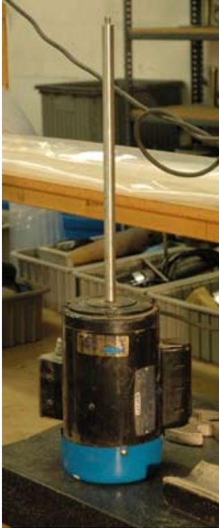
Fig. 1. Position Motor/Shaft Assembly as shown. Secure Assembly, then turn on Motor to determine if Shaft is balanced or unbalanced.
