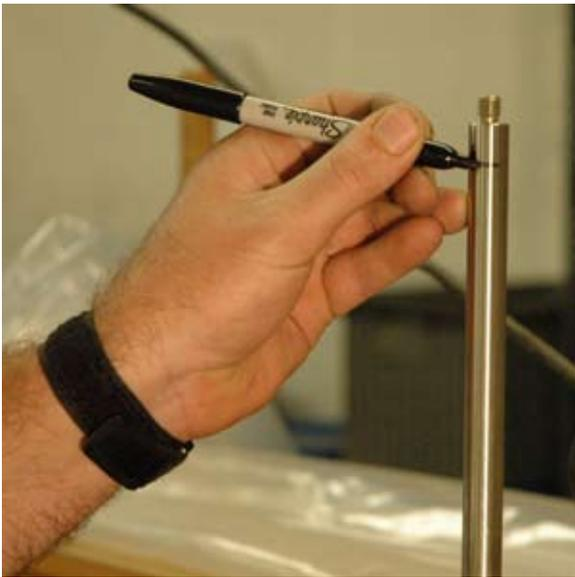
Fig. 4. With Motor on, lightly hold felt-tip pen about 1 inch (25 mm) from threaded end of Shaft.
