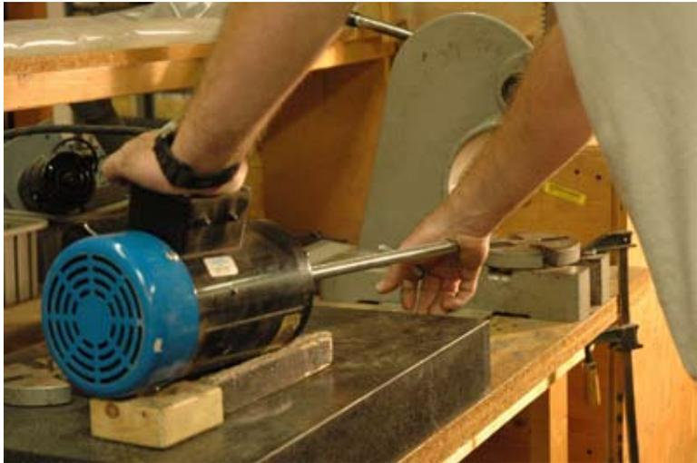
Fig. 3. Put one hand firmly on Motor to stabilize Assembly. With other hand, push down firmly on "high" spot on Shaft.
