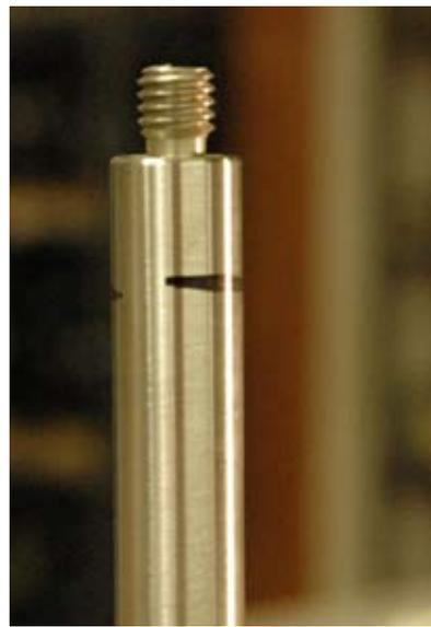
Fig. 5. If Shaft is out of balance, pen mark will be broken (not a complete circle), as shown.
