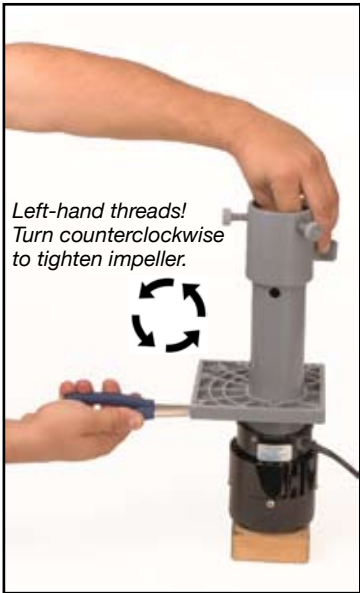
Fig. 7—To reinstall, use needle-nose pliers to hold Shaft. Turn Impeller counterclockwise to tighten.
