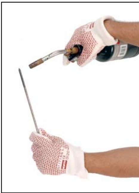
Fig. 10—Use torch to heat one end of ice pick or similar metal object.
