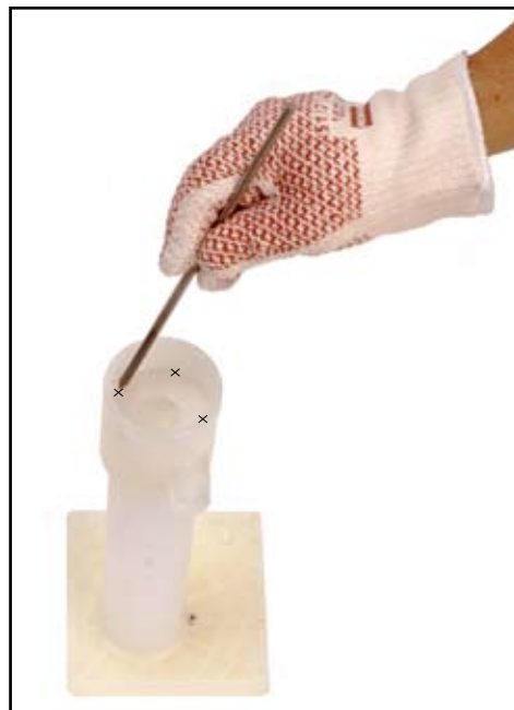
Fig. 11—Touch hot end of object to three locations shown above. This will "weld" Flow Plate onto pump body.
