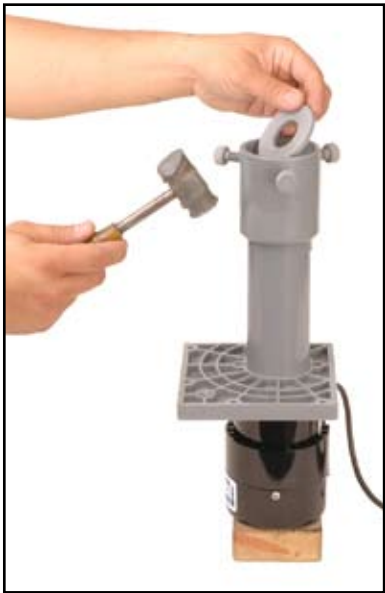
Fig. 8—Reinstall Flow Plate by lightly tapping with hammer. Then turn pump on to make sure it operates properly.
