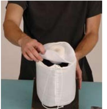
**Fig. 4. Lower Ring to bottom groove of Permacore Head.**
