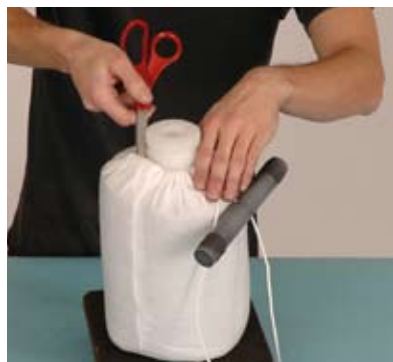
Fig. 9. Use pointy tool to move bag material close to Head.
