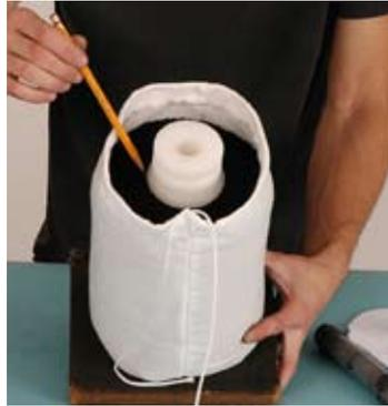
**Fig. 2.** Fill with carbon to bottom of Permacore Head.
