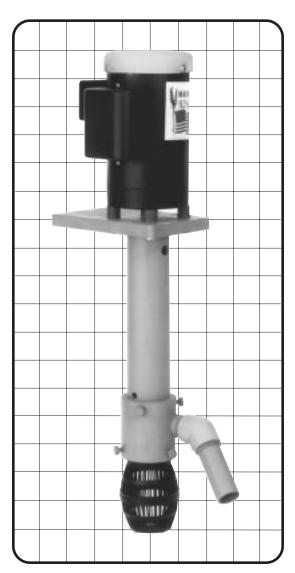
When used solely for agitation, SP12K employs a strainer as shown in photo above. For filtration (right), SP12K includes required Super Quad Cartridge Holder and Super Slide-in Filter Cartridge Adapter (Super SIFCA). These enable operator to change the four filter cartridges without moving pump from tank. Pump discharge port, Super SIFCA, and filter assembly are easily rotated to desired location in tank.
